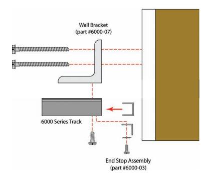
2. Attach the Wall Bracket to the wall using the appropriate mounting method (drywall & stud method illustrated here).
